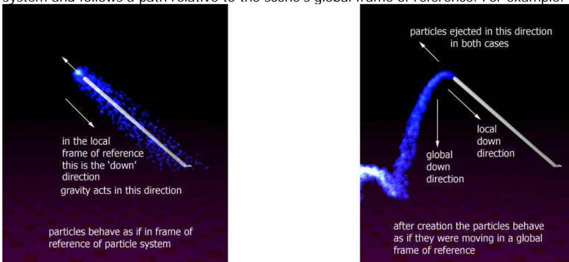
When a particle system moves during an animation the particles will keep their positions relative to the moving particle system unless this flag is set. For example in the image below we see a particle system representing a fire at the centre of the 'framework', the 'framework' which is moving from left to right.
