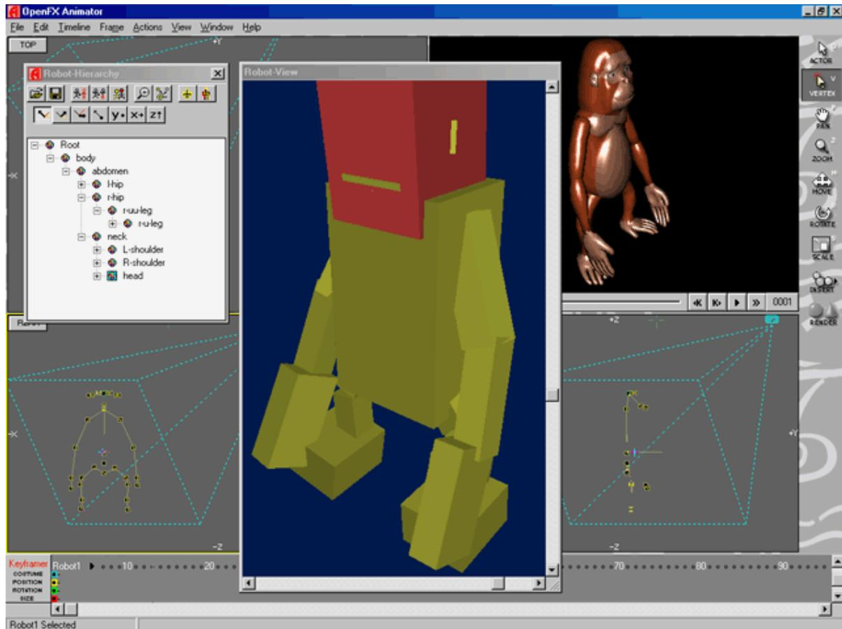
The Robot Hierarchy dialog provides a Treeview and Toolbar for selecting a Joint to pivot about and perform other editing actions. A comprehensive set of axes around which the joint may be pivoted is provided. One set of axes is relative to the hierarchical structure and the other is relative to the Robot as a whole.
