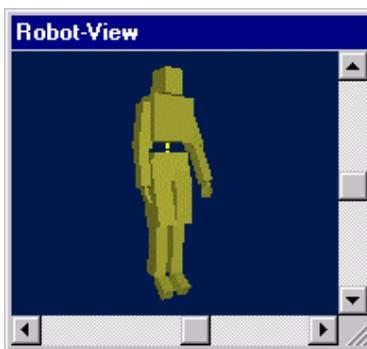
The Robot View will always be centered on the selected Robot and show it's pose. Pan the Robot-View or use the sliders to change your view point. Note that the Robot View is independent of what the Robot is doing (moving, rotating, etc.) on the stage. In the Robot View, the selected joint is indicated by a large white circle and the axis about which that selected joint will pivot is shown as a white line.
